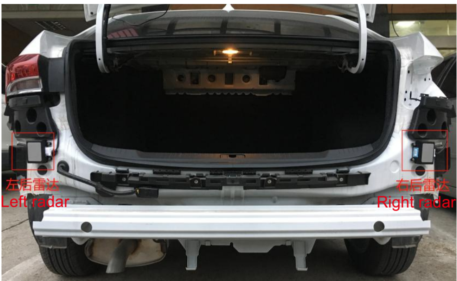
Physical Diagram for Installation Position of Radar
